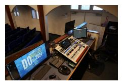
board to the Behringer Wing48. This advanced audio console offers enhanced control, superior sound quality, and greater flexibility for our audio engineers, ensuring an optimal audio experience during services.
